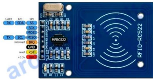
Module RFID-RC522 Arduino datasheet, pinout
